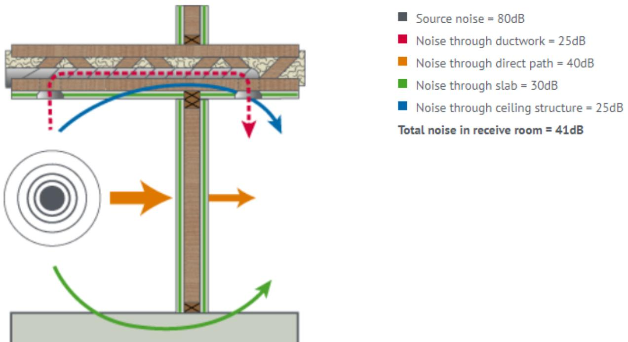
This diagram illustrates the importance of considering the entire system by showing some simple flanking noise paths that bypass a door or wall. The red arrow is direct sound – what you would measure in a lab test of a door or wall to arrive at an STC rating. The green, orange and blue paths are some simple “flanking paths”. These paths are often more important than the direct, red, path because of the effect they have on the system performance.
